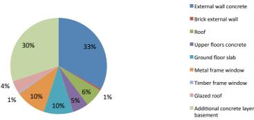
As an example, the above graph shows the relative impact of each building element in the total embodied carbon for the 30 Brompton Square subterranean extension.
