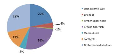
As an example, the above graph shows the relative impact of each building element in the total embodied carbon for the 36 Markham Square extension.
