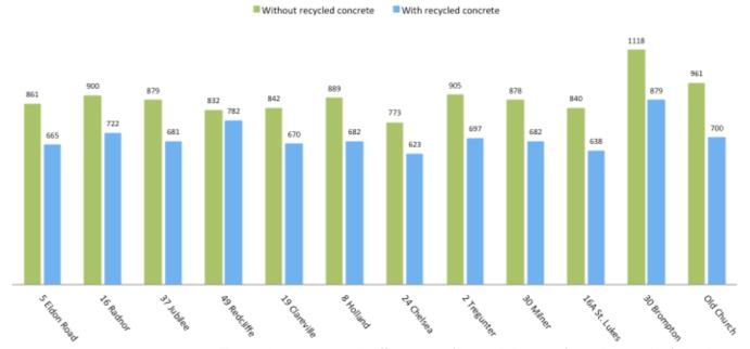
The graph above shows that if concrete with recycled content is used, the embodied carbon results over 60 years are likely to be reduced by approximately 19% for single storey basements and by approximately 23.5% for multi storey basements.
