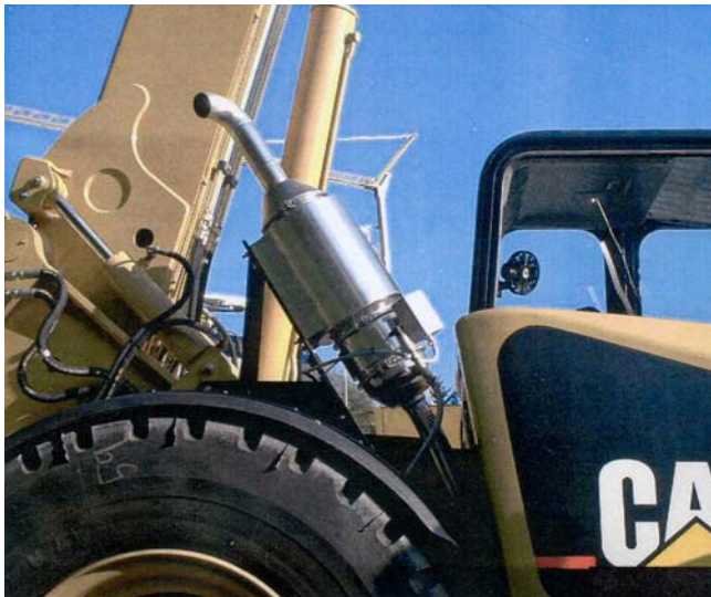
Figure 5 Diesel particulate filter (DPF) fitted to plant exhaust. Courtesy of Johnson Matthey
