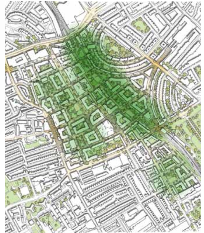
Figure 1.27: Illustrative plan demonstrating how much of this Scenario is within 100m walking distance of a public green open space
