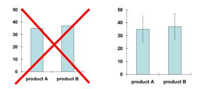
The diagrams above show the appropriate interpretation of a LCA. Note that a unanimous conclusion is not the aim, the aim is to demonstrate a range of potential outcomes.
