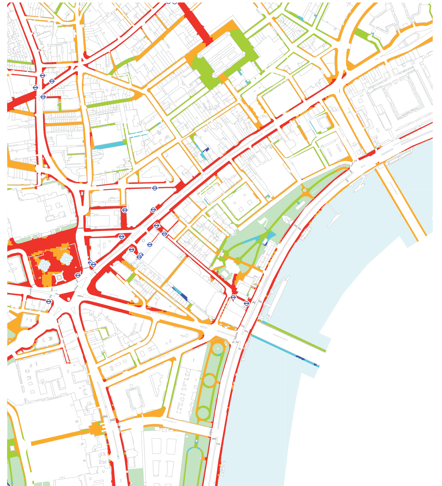
Figure 12 Example of underground station accessibility for central London. High accessibility is shown as red, moderate accessibility is green and low accessibility is blue.
