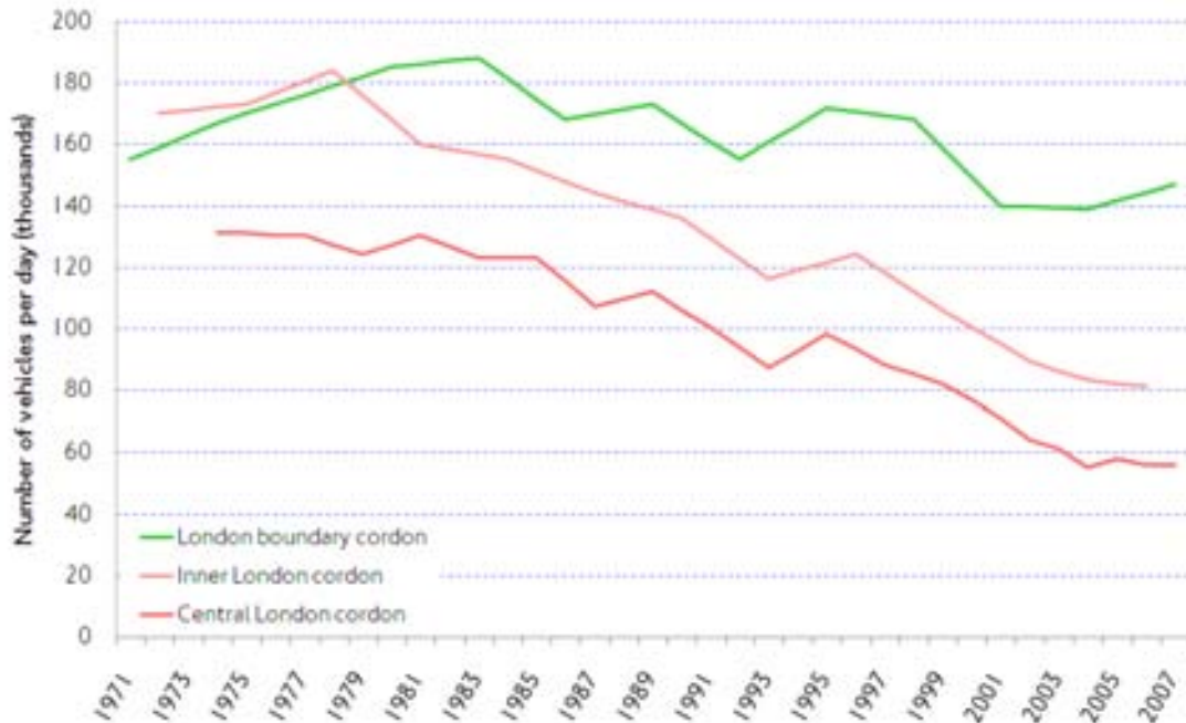
Figure 8.4 Long-term trends in goods vehicles across three strategic cordons in London: heavy and medium goods vehicles (24-hour weekdays, both directions)
