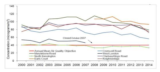
Figure 12: Exceedences of the annual mean NO<sub>2</sub> objective in the borough (Marylebone Road in the City of Westminster is shown for comparison purposes) (Source: RBKC Air Quality and Climate Change Action Plan 2016-2021)
