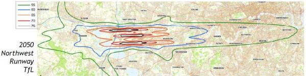
Modelled noise contour mapping commissioned by TfL and carried out by CAA's ERCD consultancy, showing the possible eastward extent of the 55 dB Lden footprint using certain assumptions, and covering the lower half of Kensington and Chelsea.
