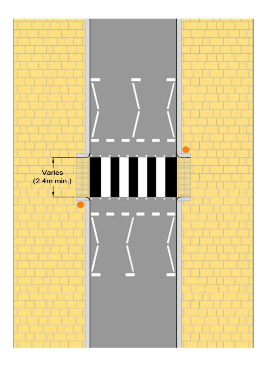
Minimum number of zig zag markings to be used. Number may be increased where site conditions dictate Belisha beacons to be mounted on lamp columns where appropriate
