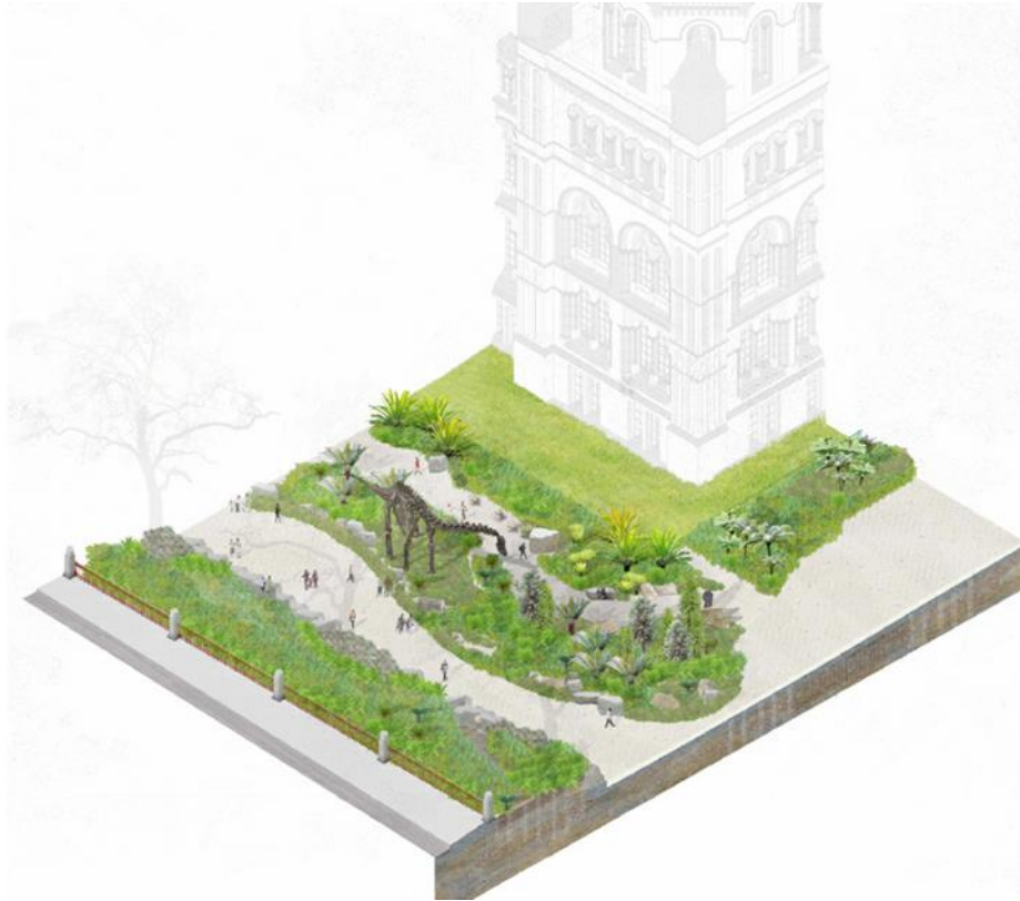
Figure 12.6: Grounds of the Natural History Museum SuDS proposal. It includes a range of SuDS measures including dry and wet swales, ponds, and permeable surfaces.
