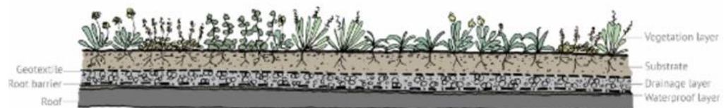
Figure 11.4: Green roof section profile (Susdrain website 59 ).
