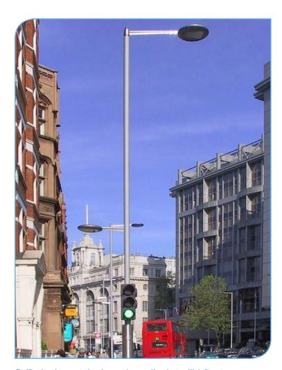
Traffic signals mounted on lamp column — Kensington High Street
