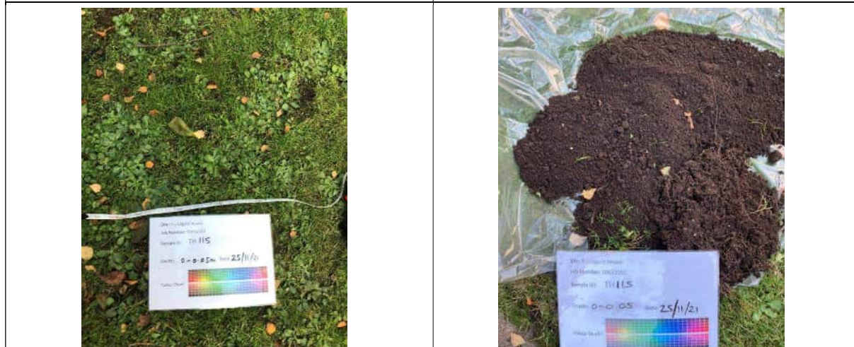
Photo 3: Excavated soil ready for sampling (0.1-0.2m) Photo 4: Excavated soil ready for sampling (0.3-0.4m)
