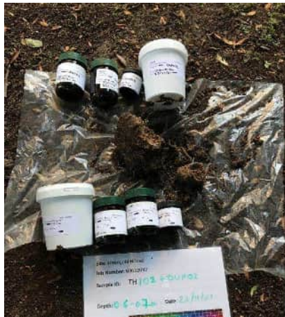
Photo 9: Sample collected in containers (0.6-0.7m) (note, error in sample location on photo board, DUP02 was not taken at TH102)
