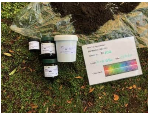
Photo 9: Sample collected in containers (0.6-0.7m) (note, error in sample location on photo board, DUP02 was not taken at TH102)
