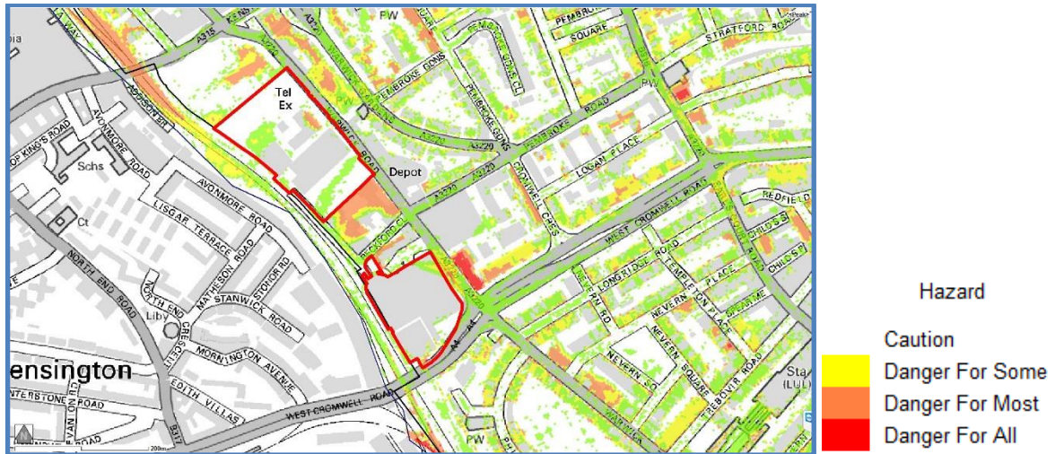
Figure 8: Surface Water flood depth (top) and flood hazard (below) of the Warwick Road Sites strategic site.
