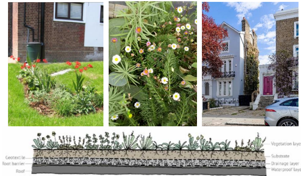
Figure 3: from left to right and top to bottom: rainwater garden ( Susdrain website 1 ), green roof on Acklam Road Mosque, green wall at 32 Kensington Park Road (photo credit: photoBECKET) and green roof section profile ( Susdrain website 2 ).
