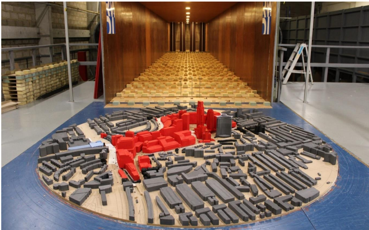
Figure 7.2: Wind Tunnel Model of Proposed Development and Surroundings
