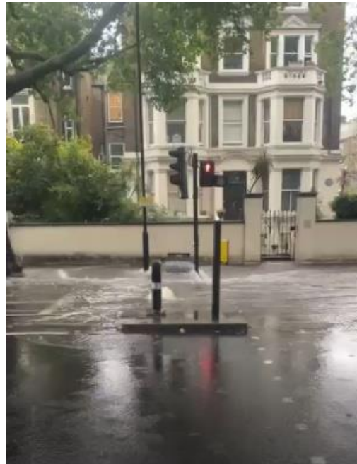
Figure 9-1: Surface water flooding which can be made up of pluvial (rainfall) and sewer flooding from surcharged sewers (images reproduced from residents' response to the RBKC questionnaire). Left: Lower Clarendon Walk; Right: Holland Park Avenue.
