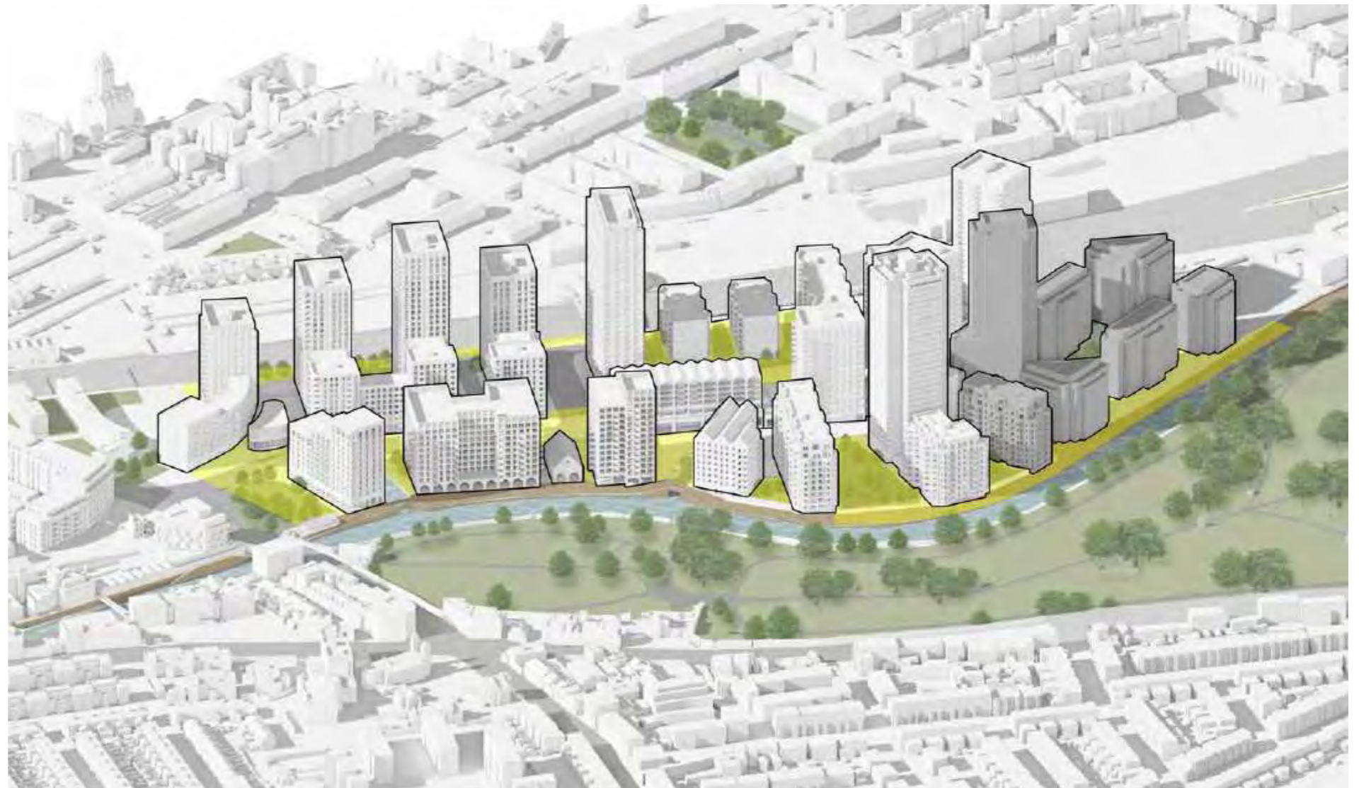
Fig 3.101: A diagram to show the principle of gaps and steps in building mass to provide day lighting at ground level.
